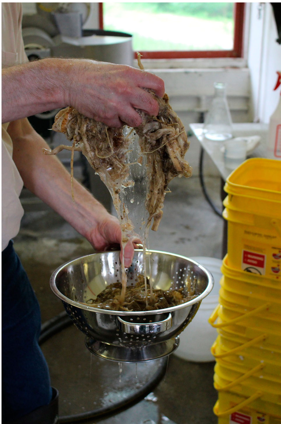
Figure 4. Neri , viscous mucilage formed when smashed roots of Hibiscus manihot are introduced to water.
