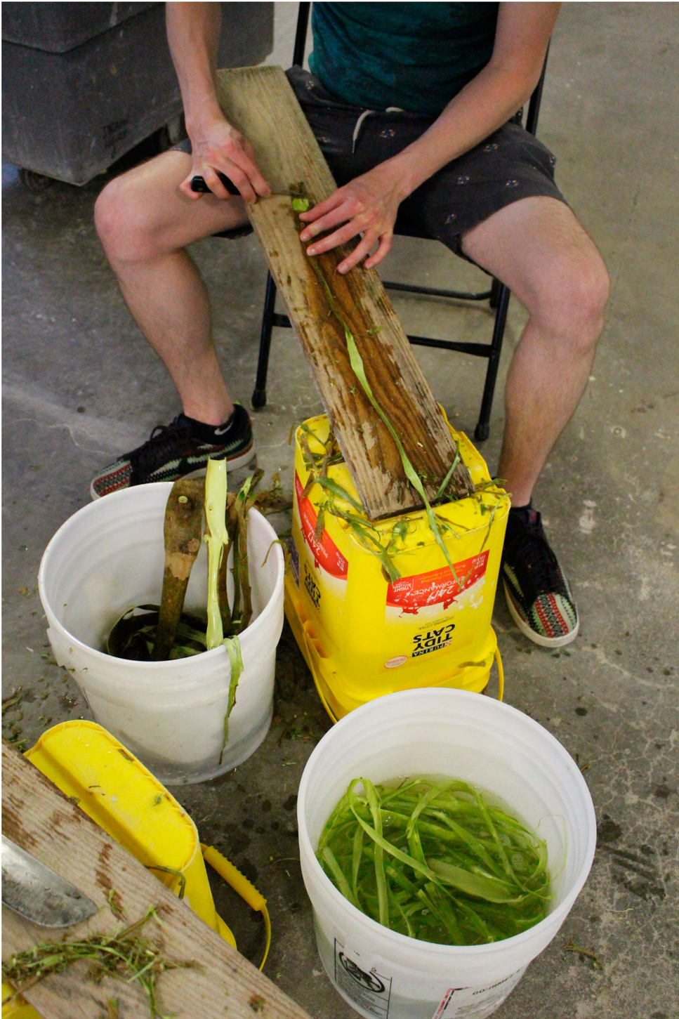
Figure 3. Removal of black bark. Left bucket: bark tissue with outermost layer (black bark). Right bucket: green and white bark.
