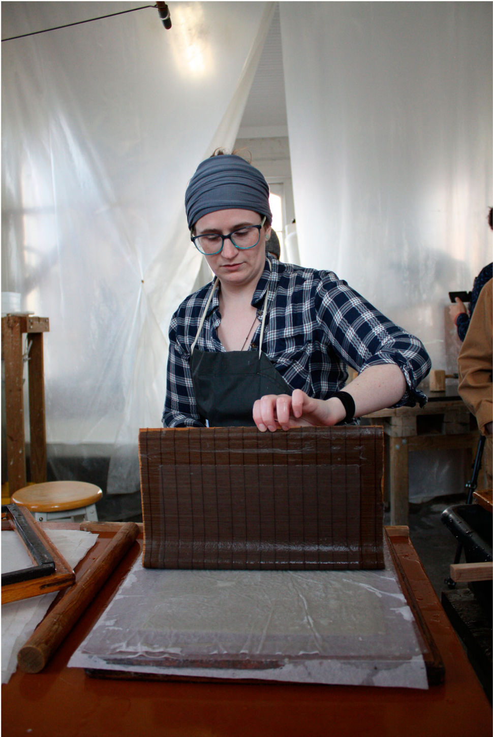
Figure 9. Couching of a sheet of Dirca mexicana paper onto a sheet of felt.
